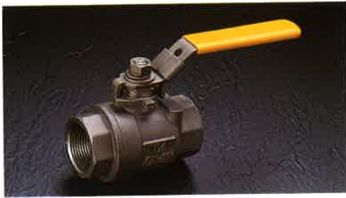
Fig. 2F124T, 2F133T 1000PSI Investment Cast 2PC Ball Valve Full Bore
